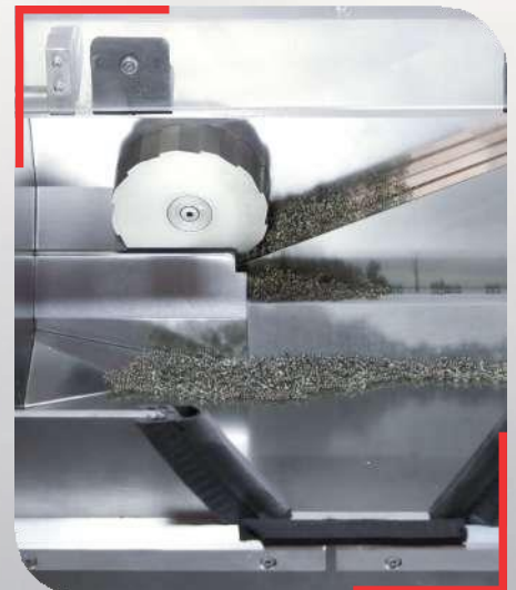
The detangler easily handles small, medium and large springs.
