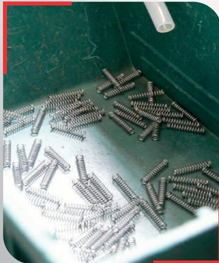
The springs can be distributed to various outlets on rails or belts.
